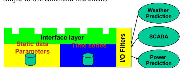
All data is stored centrally in two data bases: static data and parameters (bottom, yellow), and time series data (bottom, blue). The implementation and the data bases itself are hidden by an interface layer which provides standardised SOAP web services to store and access data (light green layer). These data management structures communicate with the outside world via I/O filters yellow, right. Data can be transported via email, sftp or SOAP/https
