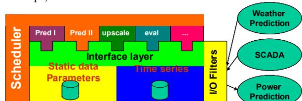
*The system operation is controlled by a scheduler task (left) which is configured via the user interfaces.*
